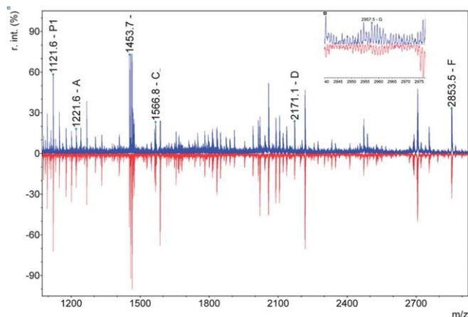
**Fig. 8** Peptide mass fingerprints from the Yup'ik kayak deck strap and covering (blue, top) and bearded seal reference (red, bottom). Bearded seal markers from Table 1 are indicated in the Yup'ik kayak fingerprint. Bearded seal is unique among Phocidae with a 1121 Da A-ion and could be identified exactly among our references. G-ions (inset) are from the unfractionated samples.
