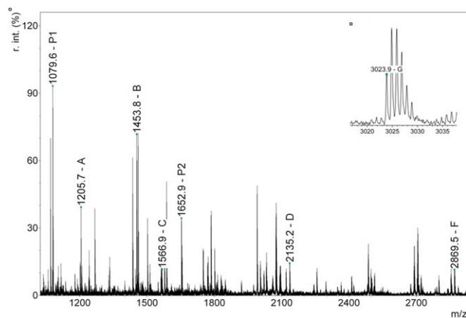
**Fig. 11** Peptide mass fingerprint from the Alutiiq kayak stitching identified as humpback whale based on marker ions in Table 1. Humpback whale can be differentiated from the other baleen whales in Table 1 by the 2869 Da F-ion. The G-ion is from ZipTip® Fraction 2.
